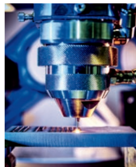
Close-up view of the wire LMD with coaxial ring beam. Source: Fraunhofer ILT, Aachen, Germany / Volker Lannert.
