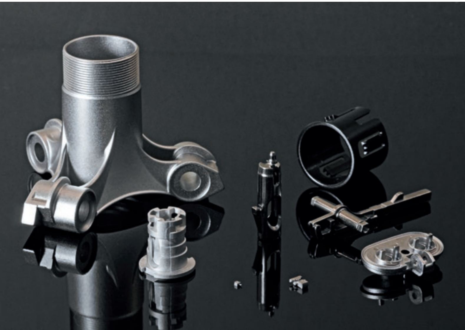
Photo on top: A selection of Metal Injection Moulded parts showing the range of shapes and sizes that can be manufactured by the technology, typically to net shape. The smallest part here is a 316L stainless steel locking device for a spectacle frame hinge, weighing 0.028 g and produced in volumes of more than 4 million parts a year. The largest part is a 316L tripod base which weighs 260 g and is 65 mm high. Source: PIM International
